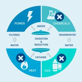
Based on the electrochemical oxidation technology, it only requires an electrical potential between two electrodes in water.
