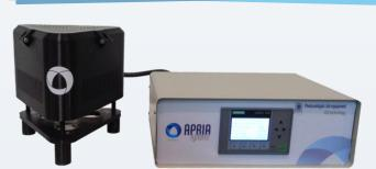
Our know-how in photocatalytic process, allowed us to design a series of flexible collimated beam equipment with LED technology. The equipment has three LED collimated beam devices with independent control and different wavelength (UV-C, UV-B, UV-A, vis or IR light can be included).
