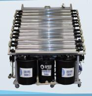
APRIA Systems built a photo-Fenton pilot plant -Photobench LED365-48/450-48a/CPC2- that can work using either a compound parabolic concentrator (CPC) solar reactor or two LED annular photoreactors. The source of light of the photoreactors are comprised of UV-a and vis LED of adjustable intensity and refrigeration through forced air convection.
