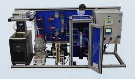
APRIA Systems integrated photocatalysis and electrochemical oxidation in one equipment. The system consists in an annular photoreactor **Photolab LED365-16/450-16a**, with UV and vis LED of adjustable intensity; and an electro-oxidation cell **ELOXlab B-S210**, with BDD anode and stainless-steel cathode. Moreover, it includes continuous online measurement of pH, T, and O<sub>2</sub>.
