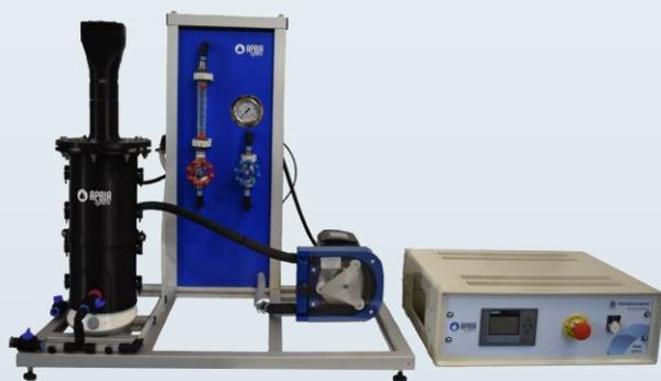
Development of a new photochemical set-up for research purposes at laboratory scale. It includes a CSTR photoreactor Photolab LED275-4c with UV-C LED technology with adjustable radiant flux and refrigerated through forced air convection. The equipment also contains an electrical console to control the lamp and a dosing pump that allows to work in continuous.
